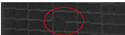
Clogged Nozzle: When the horizontal lines have small or minor gaps -- --
