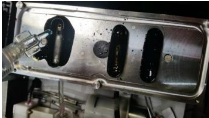
Figure 9.3-11: Flushing the Maintenance Station
