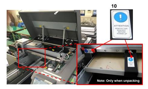
10: Remove the part indicated by the label before the machine is first turned on. Otherwise, there is a risk of damaging the machine.
