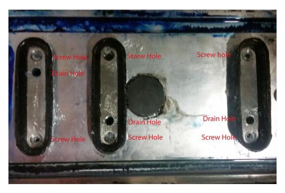
11. Secure the gaskets with *new* sealing screws, finger tight, and remove an grease blocking the gasket drain holes with the needle. *Over tightening sealing screws can break the o-ring and result improper sealing*
