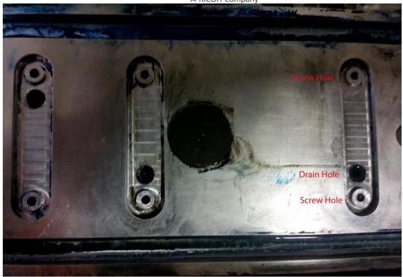
**6.** Apply grease to the gaskets slots and spread evenly across the entire surface with a narrow cleaning applicator. Failure cover the entire surface evenly could lead to a bad seal and poor suction.
