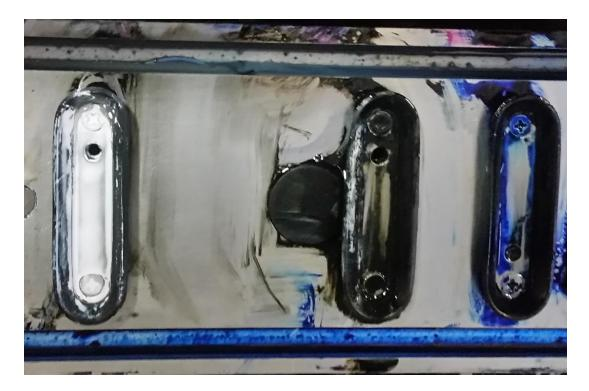
3. Remove the Philips sealing screws in the gaskets, two per gasket. Then remove the gasket and the gasket retainer
