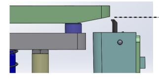
When removing the Wiper Blade please note the curved edge (lip) should be facing the Printhead Carriage when placed back into position
