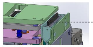
Before using the printer each day, confirm the motion of the Wiper Blade and Maintenance Station. Lubricate if not moving.
