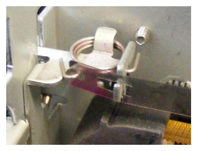
7. Lastly attach the right hand side of the encoder strip on the right hand side of the printer by pulling it over the hook, exactly like you did on the first step. Use the image below as an example.
