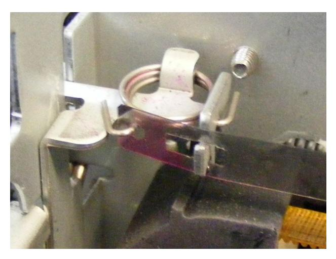
Pull the strip off the spring by pushing it towards the back of the printer and sliding it off.
