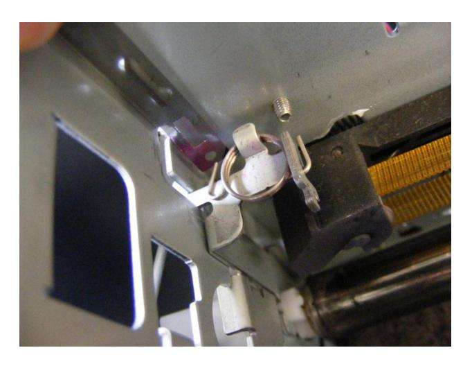
6. Now run the encoder strip through the same slot you pulled the old encoder strip out of. Before you do this, make sure you can read the numbers on the end of the encoder strip (so the numbers face you, as in the final image of this document). Now attach the encoder strip on the left hand side through the small hook.
