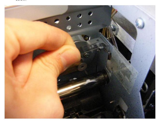
Do this by lightly pulling on the end of the encoder strip to the right and pulling it off the hook, towrds you.
