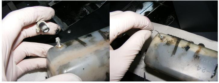
**Step 6:** If ink still does not unclog you then you may need to wash the tank out with warm water. You will need to remove the front drain tubes so that you can fill up. To remove you just need to turn the screw only two - three turns. Do not take the screw off as it holds a piece on.
