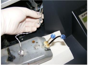
**Step 4:** You are then going to take the white clap off the drain tube. To remove you are just going to pull back to unreleased clap.
