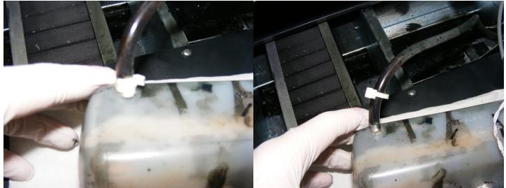
© Copyright AnaJet, Inc. 2009 All rights reserved **Step 5:** Remove the drain tube from the tank. Unclog both the tank and tube with the paper clip.
