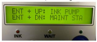
To pump ink through the system for clearing nozzles or flushing or filling the printer with ink, make sure that the Print Head is as far to the right as it can go. If the Maintenance Station is slightly to the left, it may not make an effective seal for the purpose of pumping ink.
