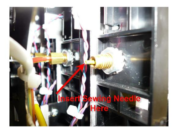
3) When finished, replace the Ink Tube and make sure that the fitting is not screwed on too tight. Finally place the ink cartridge back in the Ink Bay.
