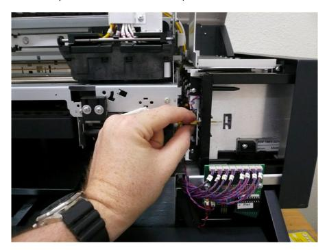
2) Place a drop of Cleaning Solution on the end of the sewing needle and insert it into the back of the Ink Needle located in the Ink Bay. Work the sewing needle back and forth, until the Ink Needle is clear.
