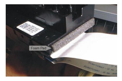
Check that the Foam Dam is properly positioned on the right guide pin.
