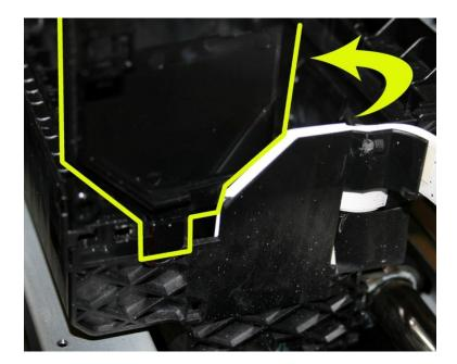
4. Remove the three M2.6 X 8 screws securing the Print Head. Lift the Print Head straight up to remove.
