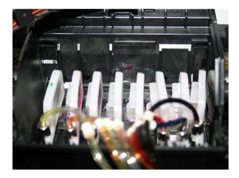
4. Before powering up the printer, make sure the Print Head is all the way to the left, then perform an Ink Charge and check for nozzle performance.
