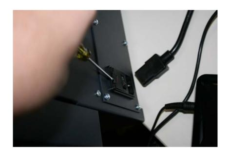
Step 2: With the screw driver remove the red fuse box.
