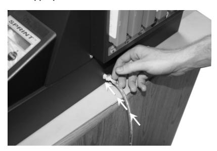
**Step 3**: Remove the Rubber Stopper from the vent hole on the top of the Waste Ink Tank and place it in a safe location. Waste ink will flow out of the Waste Ink Drain Tube.
