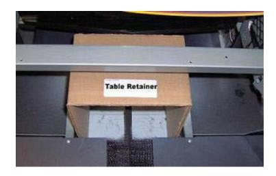
Step 9: Package the printer in the original shipping carton DO NOT PLACE ANY OTHER ITEMS IN THE SHIPPING CARTON. Handle the printer with the help of a second person to avoid damage.
