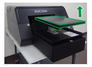
2. With the neckline of the T-shirt facing you, insert the platen into the T-shirt from the hem of the T-shirt.
