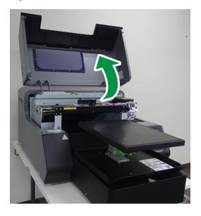
2. Wipe off any old grease and lint that are stuck on both guide rods with a cleaning applicator.
