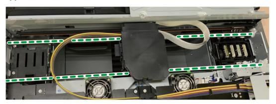
**3.** Move the carriage to the left, and then wipe off any old grease and lint on the guide rods where the carriage had stopped.
