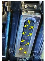
After cleaning, if washing the Cleaning Liquid and foam etc. attached to surplus have adhered to the Head, wipe it off with the dry, Cleaning Applicator that does not contain the Cleaning Liquid. (It is important not to leave wet cleaning fluid on any part of the head after this manual clean)
