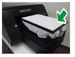
**IMPORTANT!** Make sure that the garment does not stick out of the lower frame of the platen.
