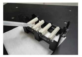
4. Take the filled cleaning liquid with the head protection cover under the carriage to prevent spillage.
