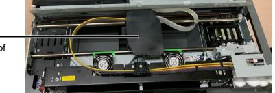
• When cleaning the guide rods, try to avoid touching the encoder or the carriage belt. This may cause the printer to not operate properly.
