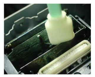
**2.** Clean the surface and the inside parts of the Wiper Cleaner.
