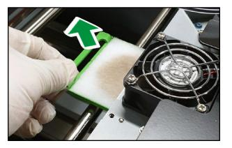
**5.** Remove the mist fan filter from the fixing frame.
