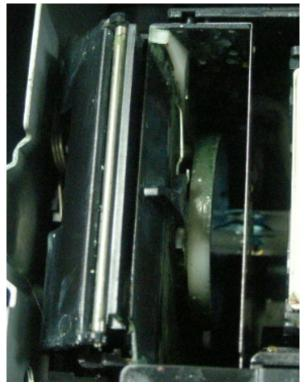
• Perform cleaning until the surface of the roller, wiper and bottom part of the wiper cleaner are completely visible.
