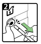
**IMPORTANT!** Do not pull the waste ink tube without pushing the plastic ring.
