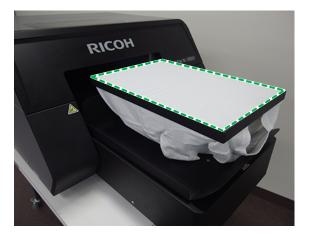
2. Adjust the height of the platen by turning the height adjustment knob under the platen.
