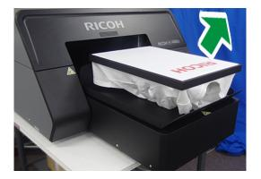
**2.** Grasp the front side of the garment and remove it horizontally from the platen.
