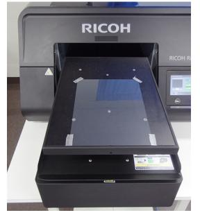
**NOTE -** Nozzle checks must be performed on transparent A4 media. If any part of the transparent A4 media is curled, tape it down to avoid an obstruction detection.
