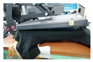
• There is a possibility that the brand or type of printed fabric is bleeding easily. If possible, change the brand or type of printed fabric.
