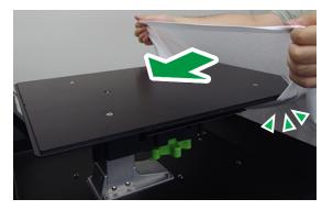
Insert the bottom of the T-shirt into the gap of the platen base.
