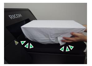
**4.** Remove wrinkles and distortion on the printed surface. If there is slack, the GAP becomes wider, so set it horizontally.
