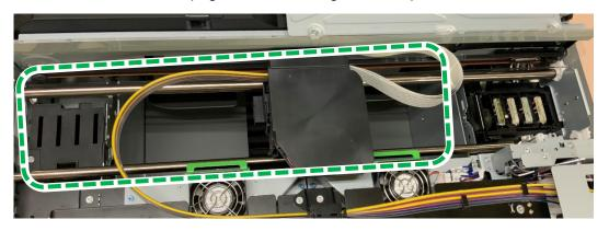
Case 2: The carriage is in the maintenance unit position. The carriage needs to be unlocked. Proceed to page 212, "Unlocking the carriage".
