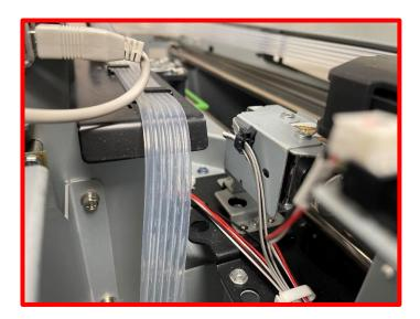
Ri2000 White lines completely clear White carriage lines should be fully clear after the 2<sup>nd</sup> flush. If you are just doing the initial flush, then the lines will still have milky appearance
