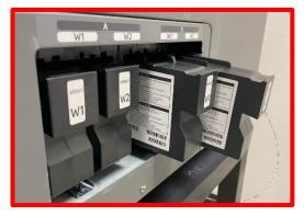
2. Remove all ink cartridges from the printer.
