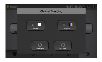
6. You have the option to flush the white carriage, the CMYK carriage, or both carriages. We will just flush the white carriage.
