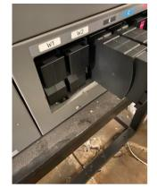
2. Remove the white ink cartridges from the printer.
